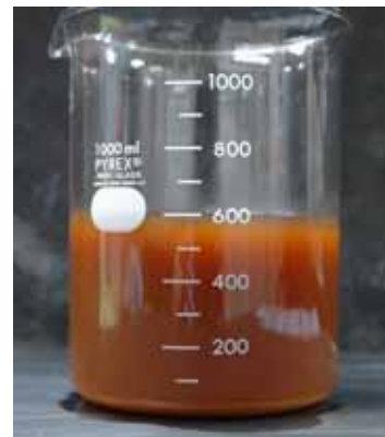
Fig.5 Representative photograph of emulsified A-Heavy oil (Water: 6 vol.% for Fuel, 800 rpm).
